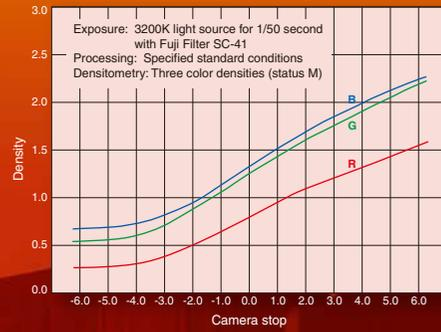
In order to simulate conditions closest to practical use, exposure was made under a 3200K tungsten light source, through a Fuji SC-41 ultraviolet absorbing filter. Processing was carried out under standard conditions and the three color densities were measured, producing the results indicated in the graph above.
